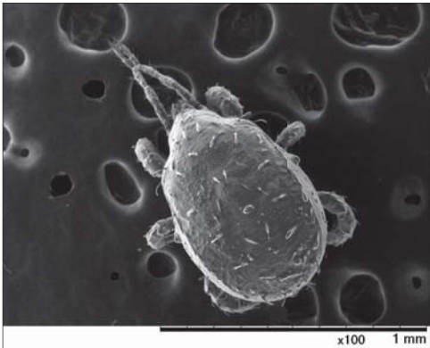
Surface (5 kV) Sample: Tick Image signal: Secondary electrons; magnification: 100x
