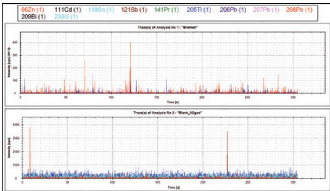
Figure 4. Time resolved scans for outside air and an N<sub>2</sub> gas blank using a 10 ms dwell time. Please note the different (vertical) intensity scales on the two scans
