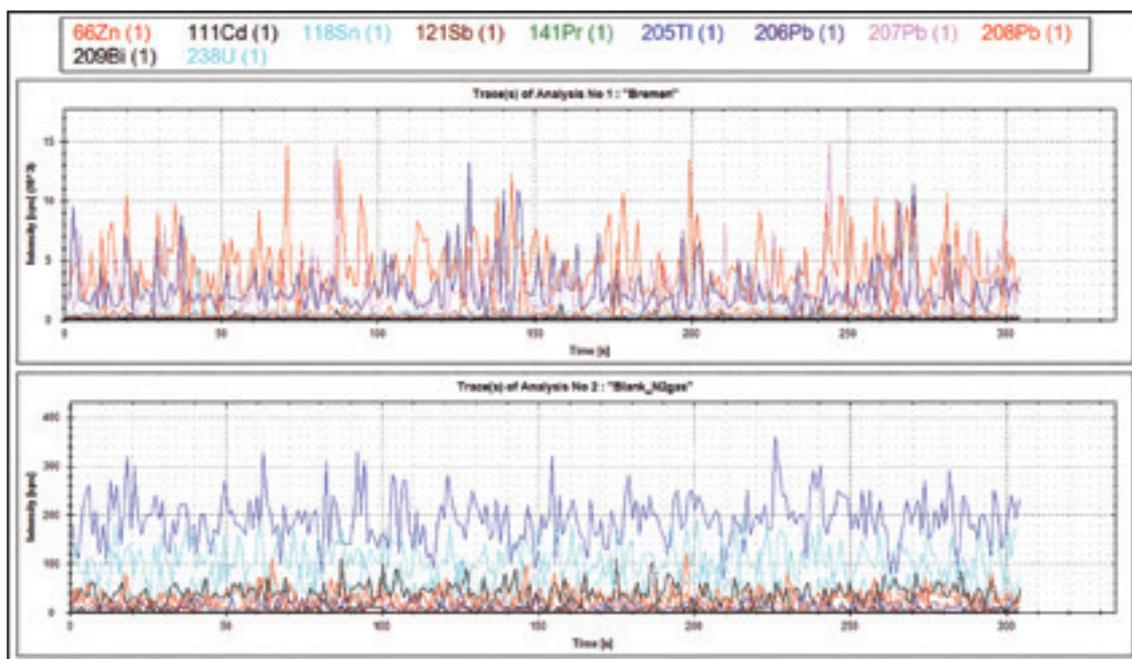
Figure 3. Time resolved scans for ambient air and an N<sub>2</sub> gas blank using a 100 ms dwell time. Please note the different (vertical) intensity scales on the two scans
