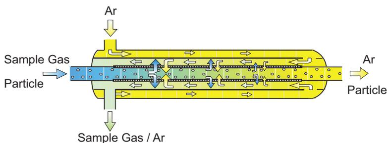
Figure 2. Principle of Gas Exchange Device
